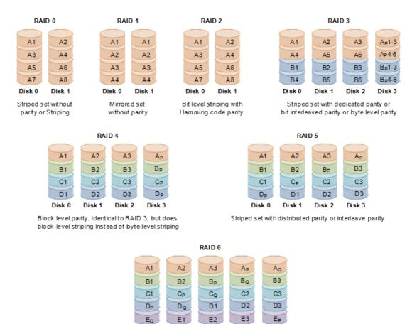
Disk 2 Striped s et with dual distributed parity
