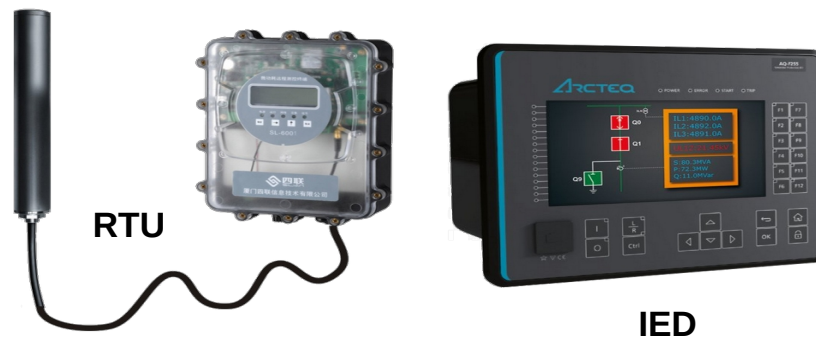
Figure 12: RTU and IED
